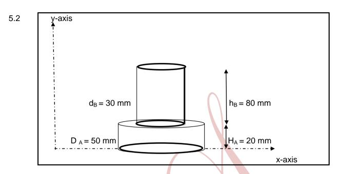
Calculate the position of the position of the Centre of gravity, y.
