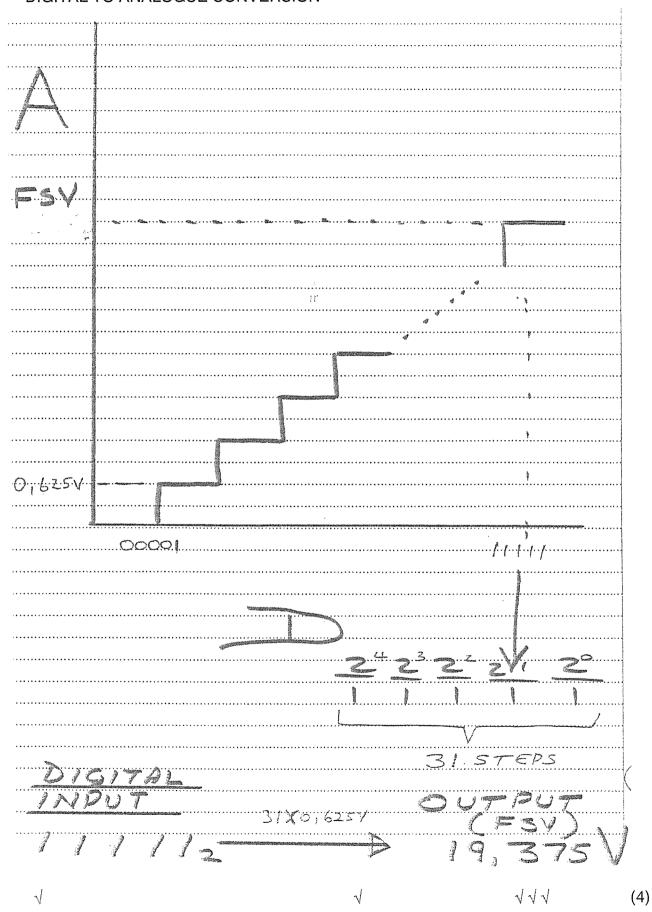
4.3 Quantizing error: As shown on the sketch below the quantizing error of a D/A converter (an ideal D/A converter where other errors are assumed to be zero) cannot be less than half the resolution (i.e. half the step-size of the converter).
